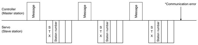
Similarly, when the master station detects a fault (e.g. checksum, parity) in the response data from the slave station, the master station retransmits the message which was sent at the occurrence of the fault. A communication error occurs if the retry operation is performed three times.
